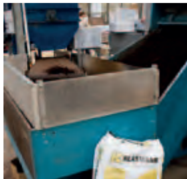
By machine (specific substrate mixers): Mixing time should be restricted to a minimum in order to maintain the structure of the product.
