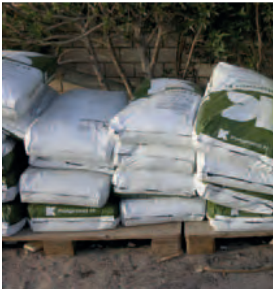
Incorrect and unprotected storage outside.
